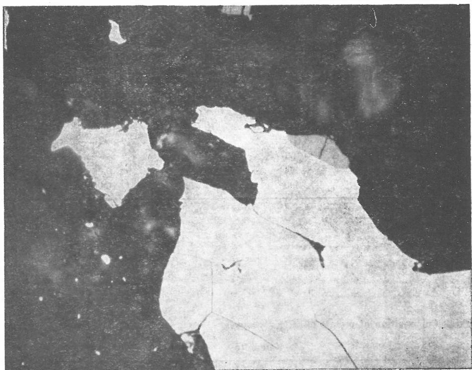
Figure 11: Small ilmenite grain growing together with troilite and metals. Photomicrograph.
