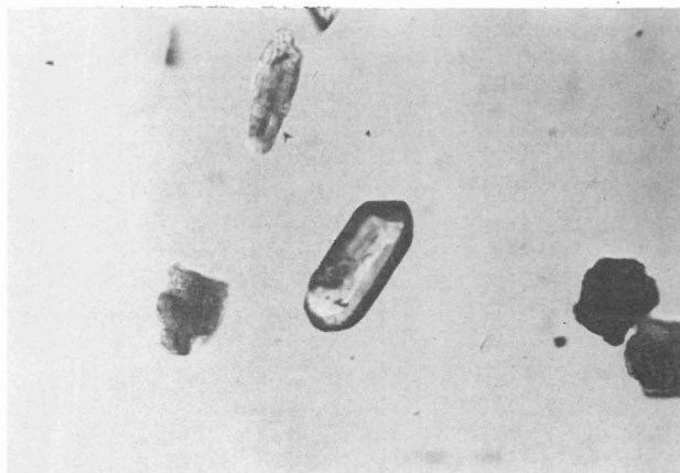
Fig. 2. Zircon — the columnar crystal with outstanding relief. From the fraction 0.063—0.10 mm of sample No. 1 from 2 nd locality Napajedla. 200× (12.5×16) enlarged.
