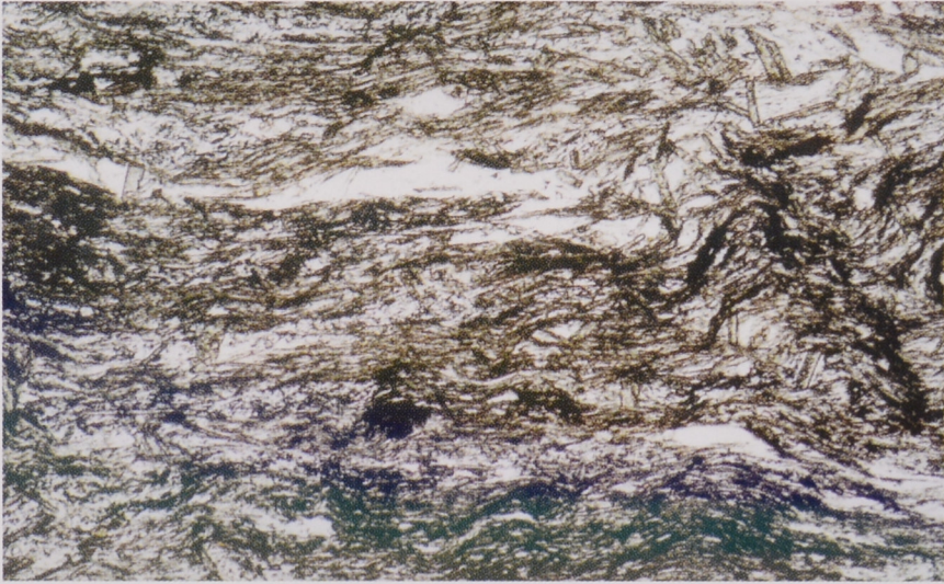
Figure 2. Translucent areas of quartz and muscovite alter pale green-brown clinocllore and paragonite. Dark areas are due to the presence of amorphous graphite. The high relief rods are of chloritoid. Same sample as above. Plane polarised light, magn. 50x.
