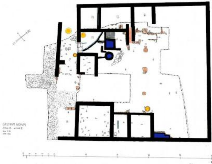
Fig. 6: The vectorisation of the handmade planimetry of the site (author: Flavio Enei). An example of the process that is carried out in IDraw. The superposition of the layer with the original planimetry and the vectorised layer (author: Klára Pačliková).
