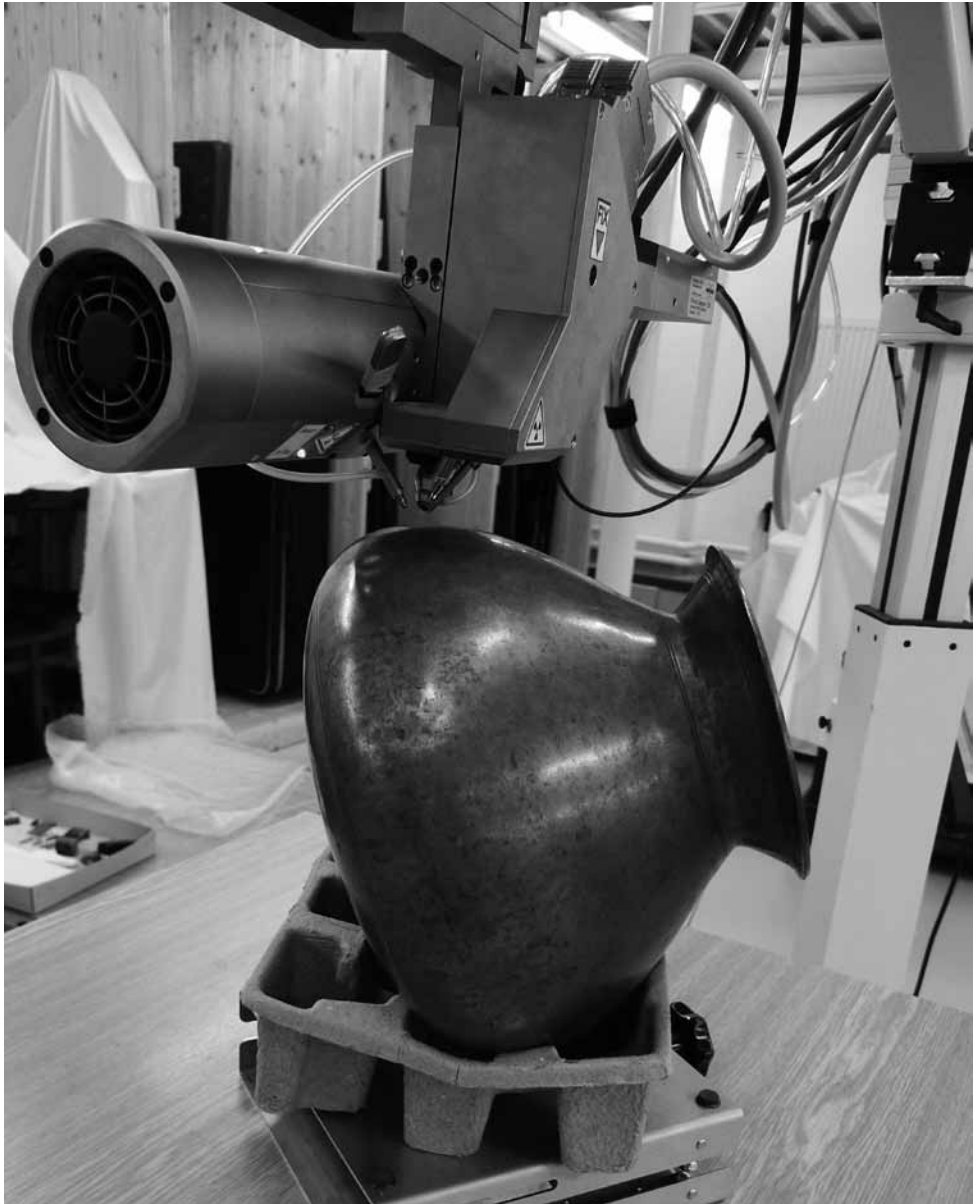
Fig. 2 Measuring a brass vessel using an ARTAX 400 instrument (photo by Michael Kotyk)
