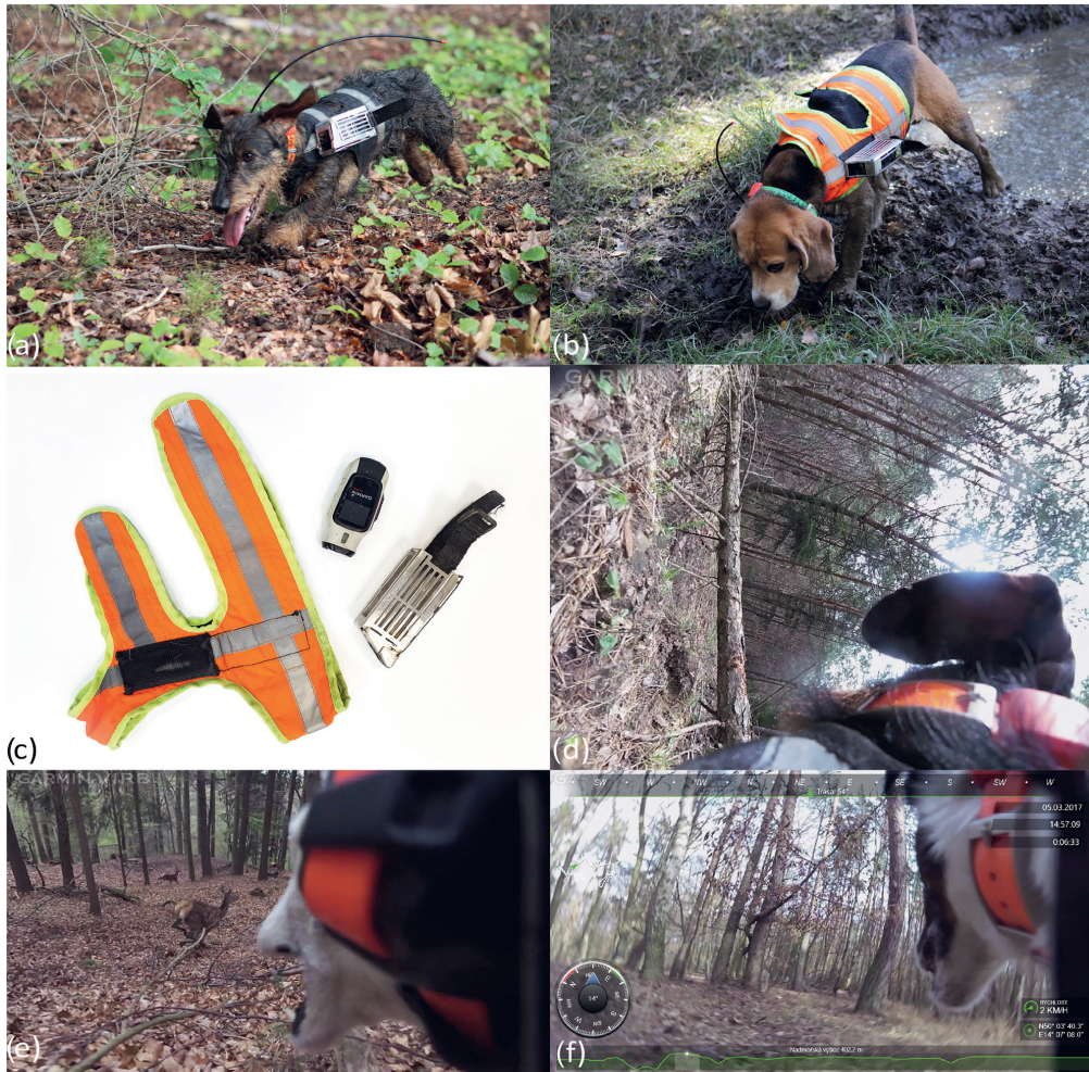
Fig. 1. Dog action camera system: (a) vertical placement of the camera, (b) horizontal placement, (c) custom-fitted harness, Garmin Virb Elite camera, stainless steel camera mount, (d) recording in 960p mode with the visible position of the dog's head, (e) recording in 720p mode, when the dog is marking the game by barking, (f) camera recording with displayed data.
